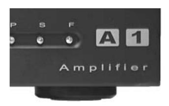
Fault/Protection: The A1 can shutdown in Protection mode for several reasons. A common reason is that the speaker output wires have shorted together. Another could be that the amplifier has overheated. Should either of these conditions occur, repairing the cause of the output short or allowing the amplifier to cool will solve the problem. To reset the A1, turn the power switch (rear panel) off and then on. If the problem persists, contact your NHT dealer.
